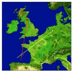
Figure 2 - Lightning Location by Triangulation
